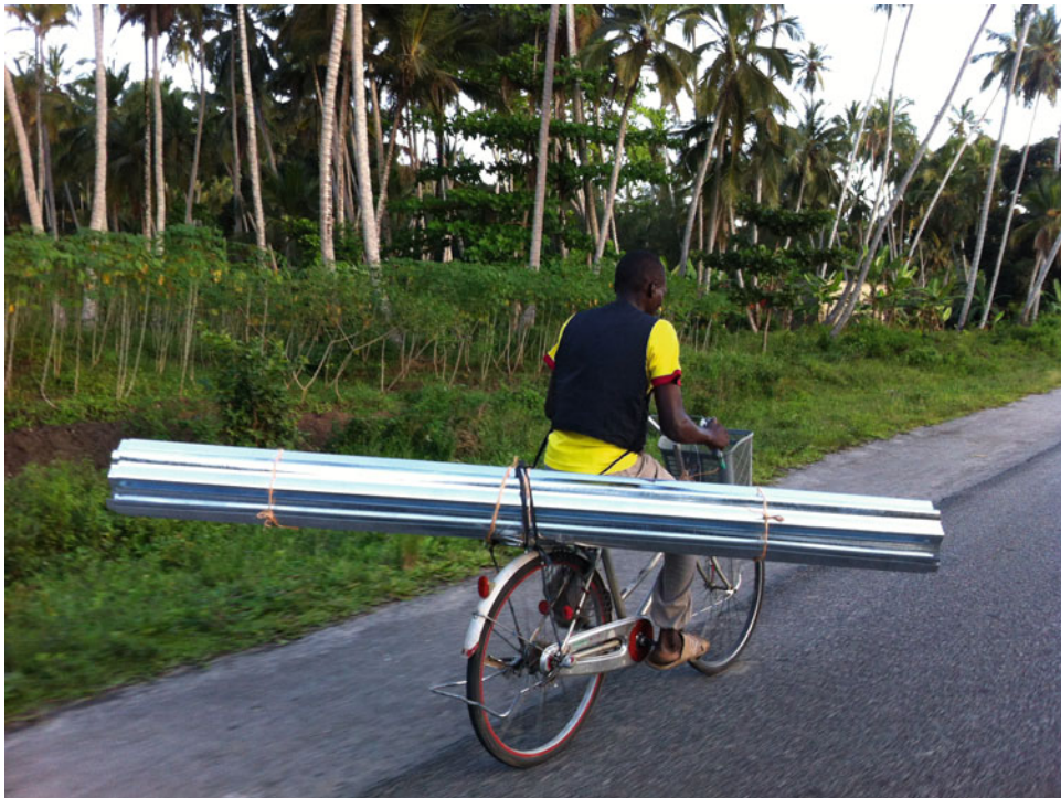
9.8 The unbeatable mabati (corrugated metal roof sheet). Cheap, lightweight, durable, easy to transport, and watertight. Photograph Muhammad Juma
